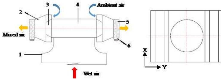
Fig. 1. Structure of plume abatement and water-saving condensing device
