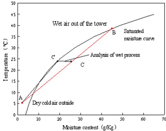
Fig. 2. Plume generation and elimination theory
