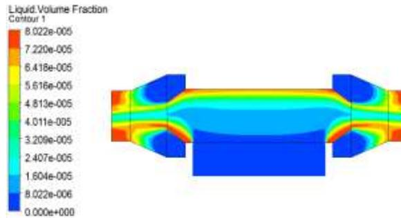
Fig. 8. Liquid water volume fraction distribution cloud of X = 2785m
