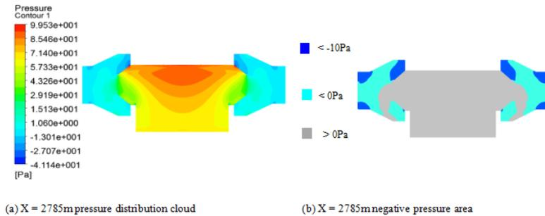
Fig. 5. Pressure distribution contours
