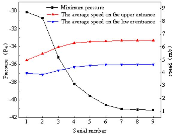
Fig. 4. device minimum pressure and inlet average speed
